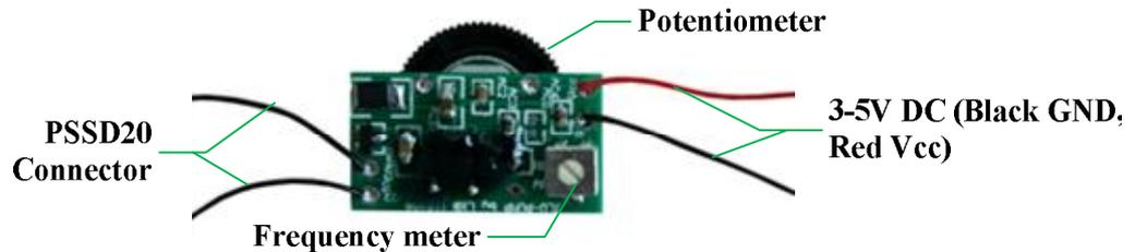
Fig.3 Piezoelectric pump micro controller
